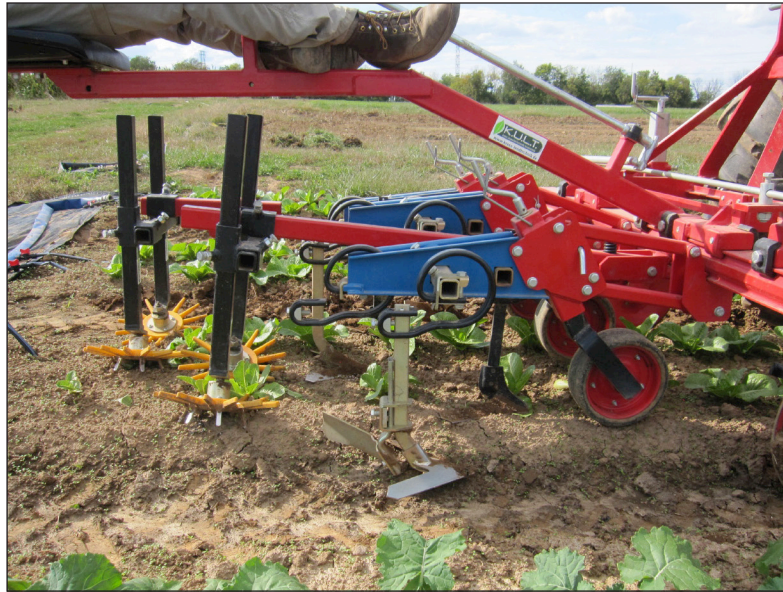
A finger weeder is being used to cultivate two rows of kale. The cultivator provides between-row and in-row cultivation at a depth of 1 inch. The yellow fingers are flexible rubber and are used to scrub out weeds in the plant rows, while sweeps and side knives cultivate between the rows and on the sides of the beds. This tool is used for the final cultivation before canopy closure and once the plants can tolerate some soil disturbance without being uprooted.
