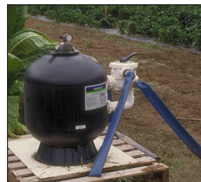
Above left: Sand filters are often used with surface water sources. Above right: Disc filters are commonly used for specialty crops on small farms in Kentucky.
