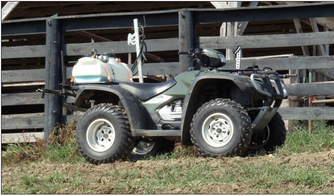
Figure 5. Broadleaf weeds were removed from the proposed filter strip area using this ATV, equipped with a spray boom.
