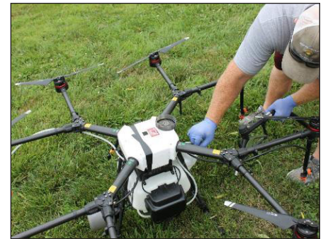
Figure 2. Drone used to apply fungicide in 2019 Adair County corn trial. Nick Roy
