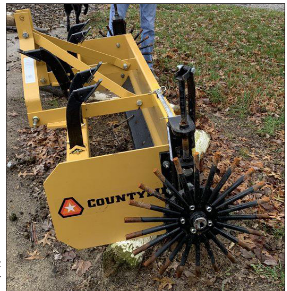
Figure 3. A box grader used to redistribute footing.
