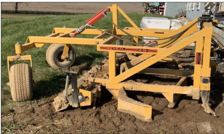
Figure 2. A multi-unit drag can be used for redistributing footing. Claire Burnham, taken at Carriage Station Farm.
