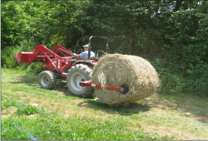
Figure 7. Clamping position for lifting bale off the ground for transport with small tractor.
