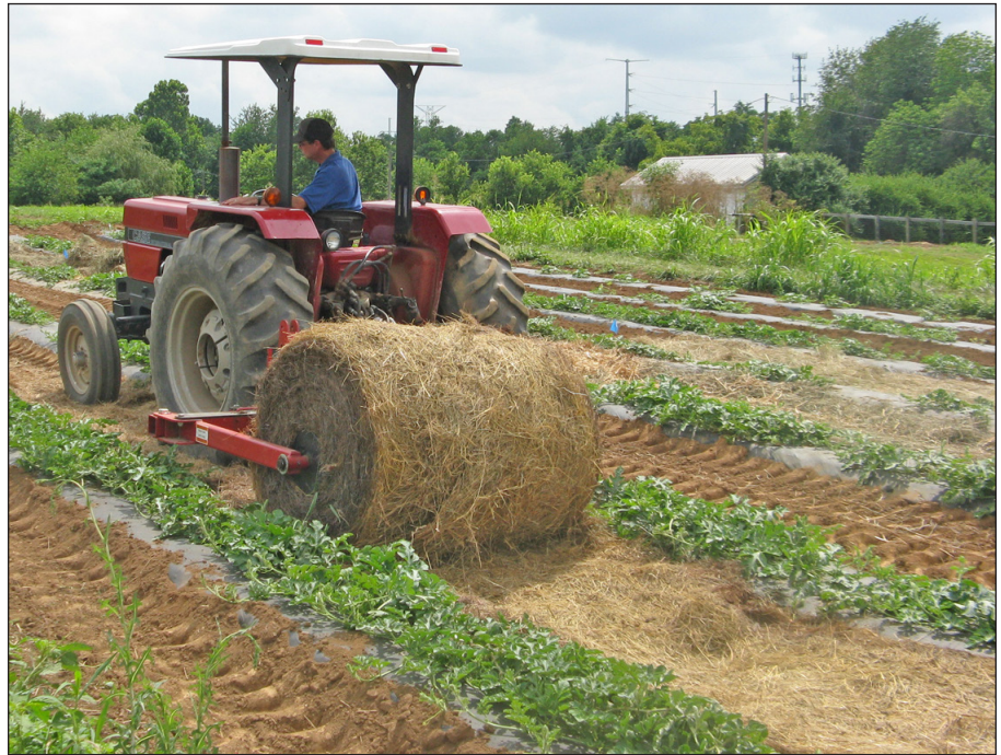
Figure 1. Offset bale unroller unrolling a round bale of hay between rows of plastic.
