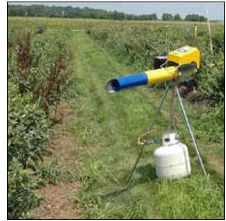
Figure 13-5. Noise makers are only partially effective, as birds quickly become accustomed to the noise.
