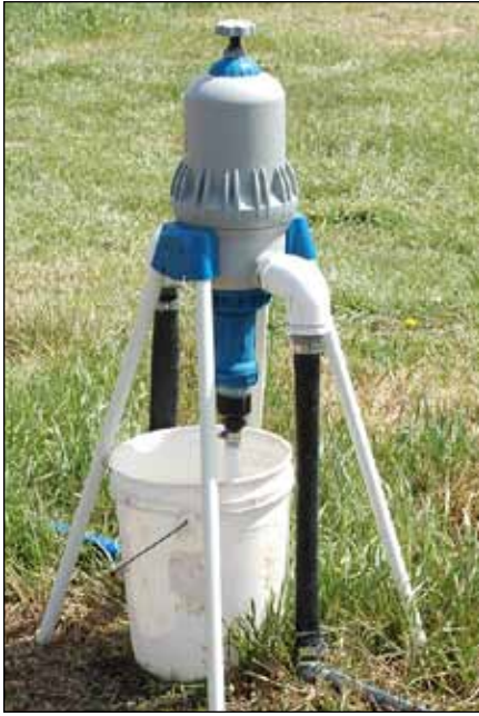
Figure 10-4. A fertilizer injector can be used to inject water soluble fertilizer through drip irrigation.
