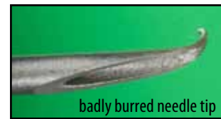
Figure 2-3. Examples of needle tips. When needles become burred they should be replaced.
