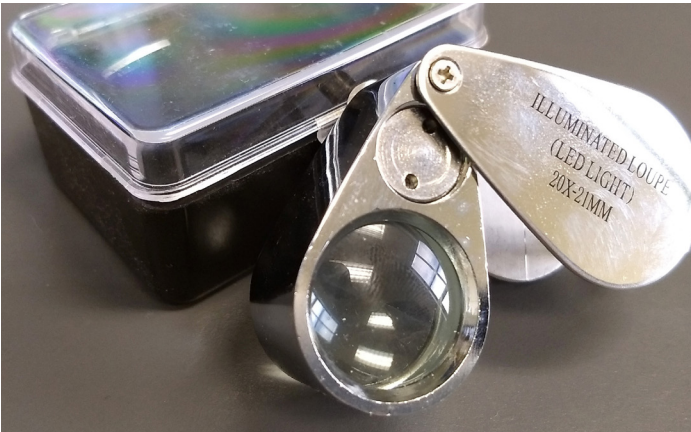
Figure 6.11. A hand lens can be used to magnify plant samples and identify signs.
