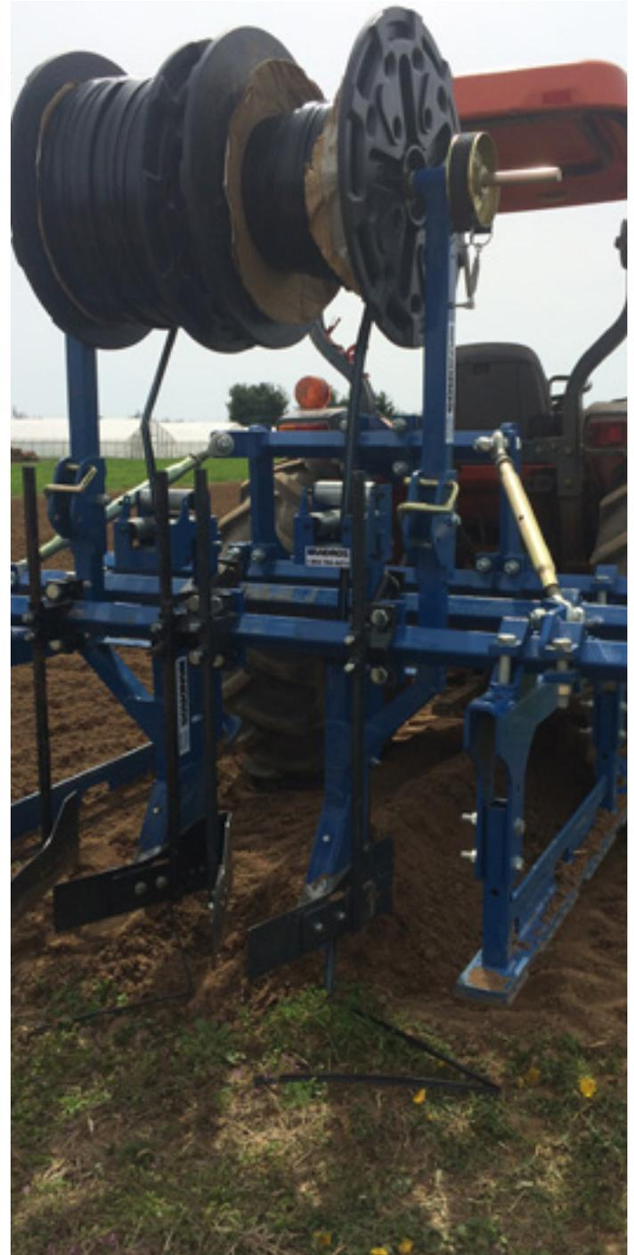
**Figure 20.** Custom Andros subsurface drip layer.
