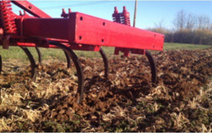
**Figure 12.** Chisel plow.
