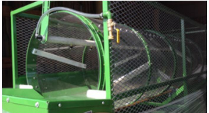
Figure 11.5 Barrel washer.
