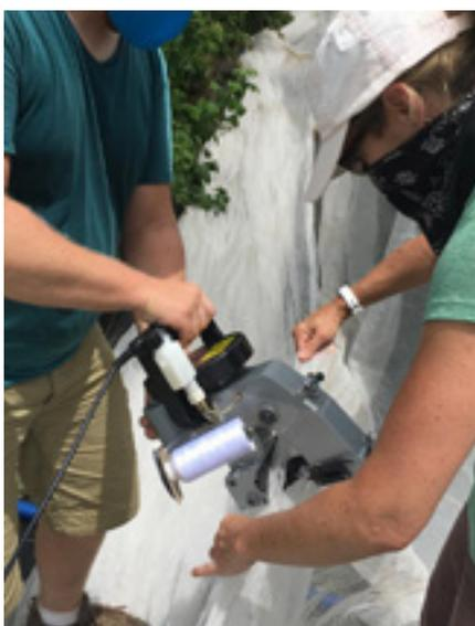
Two large pieces of ProtekNet netting are sewed together using a handheld sewing machine. Photo courtesy of Gonthier Lab.
