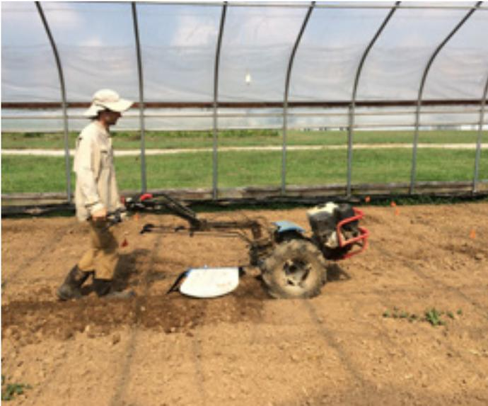
**Figure 24.** BCS rotary plow.
