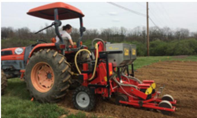
Figure 27. The MaterMacc VegiMacc vacuum seeder.
