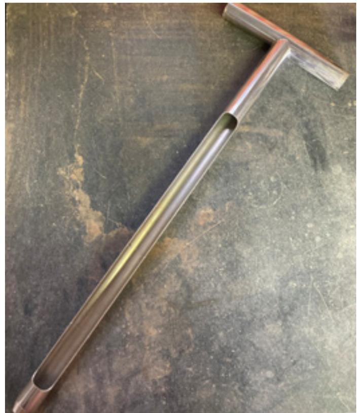
Figure 9.5 Soil probe.
