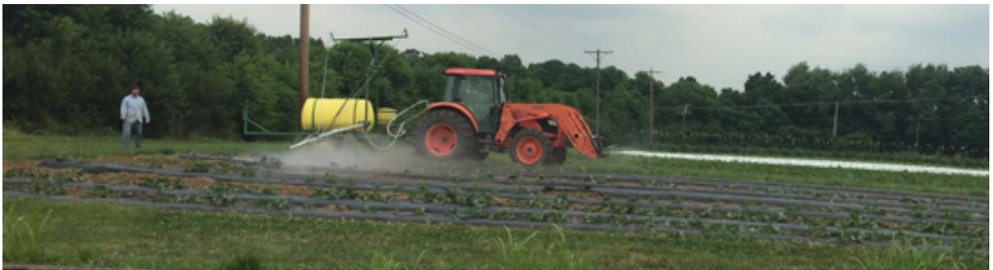
**Figure 63.** Chemical applications made with a Penn's Creek Manufacturing 25-foot boom sprayer.
