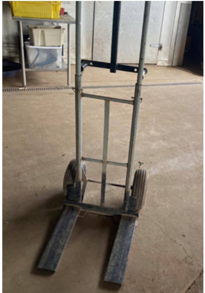
Figure 11.8 Custom hand truck with forks.
