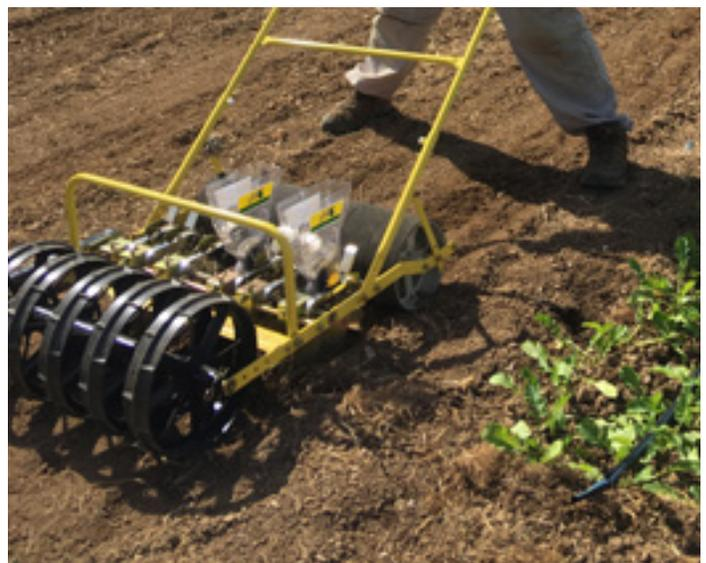
**Figure 35.** A six-hopper Jang push seeder can seed between one and six rows per bed at a time.
