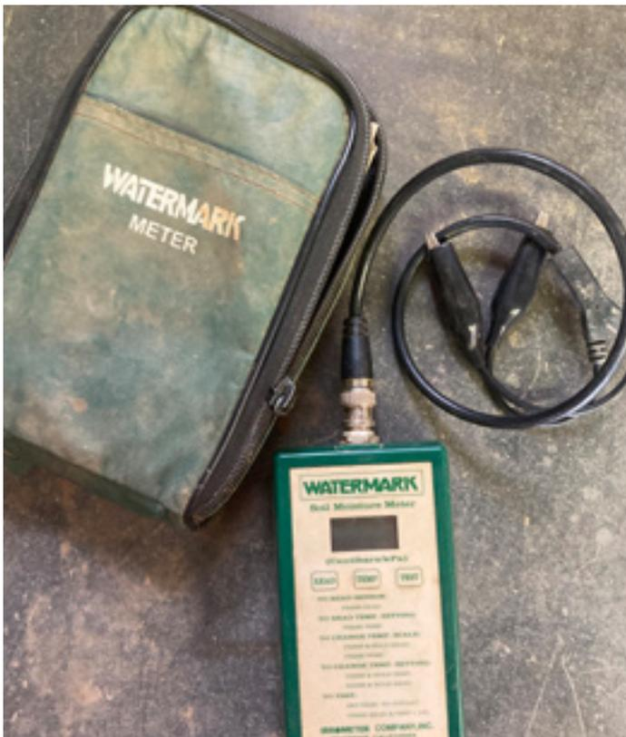
Figure 9.4 Watermark sensor meter.
