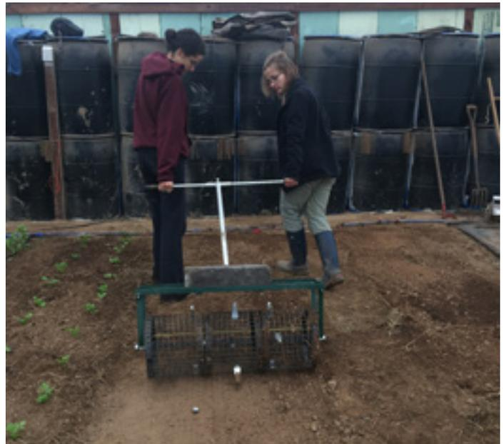
**Figure 33.** The 36-inch seedbed roller packs bed tops while dibbling holes. Dibble spacing is customizable.
