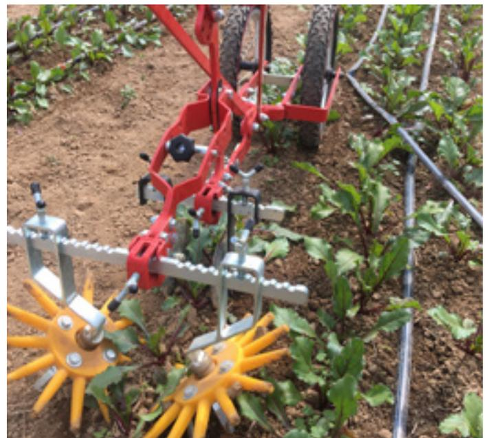
**Figure 55.** Terrateck double-wheel hoe with finger-weeding attachments.
