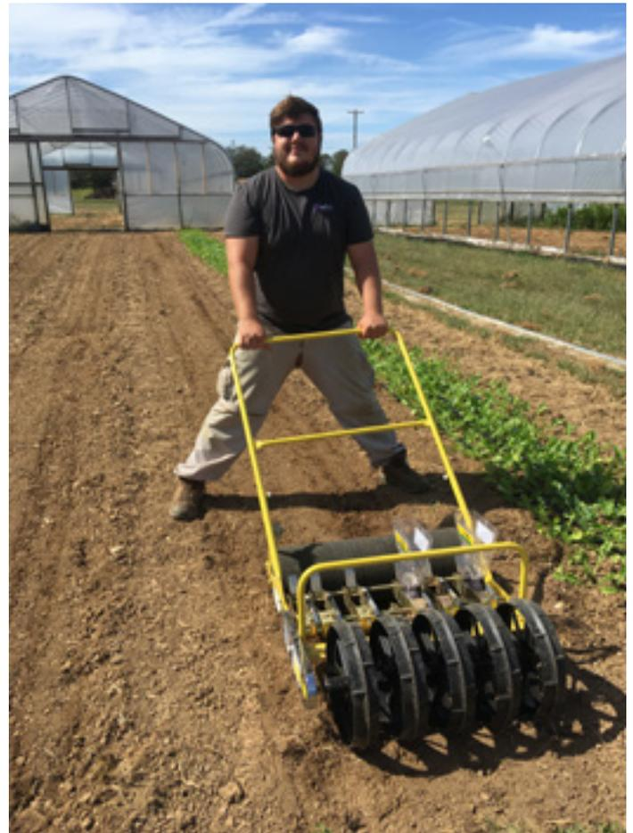
The ganged Jang JP-6 push seeder unit is heavier to maneuver, but the number of rows and spacing is customizable.
