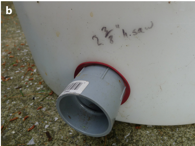
Figure 18a, b, c. Gray, 2-inch electrical conduit fittings (a) used to create a tank outlet which can be joined to standard white PVC pipe. A 2 3/8-inch hole saw was used to cut the hole in the tank (b). Different fittings are installed outside (b) and inside the tank (c).
