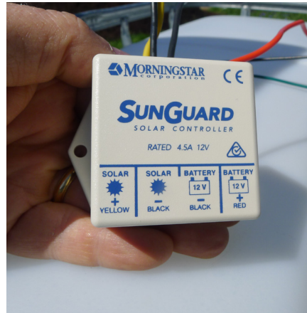
Figure 26. Small solar panel voltage controller.
