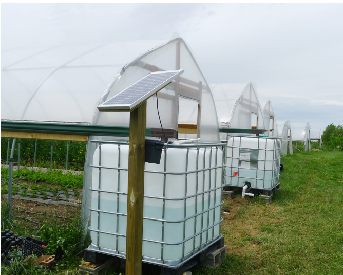
Figure 24. Tote tanks for rainwater collection from a high tunnel; the two tanks are joined by an underground PVC pipe. Drip lines in the tunnel are pressurized by gravity or the solar pump.
