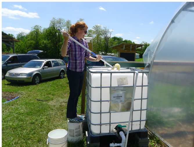
Figure 23. Cleaning a tote tank with detergent, chlorox, and a ceiling fan brush.
