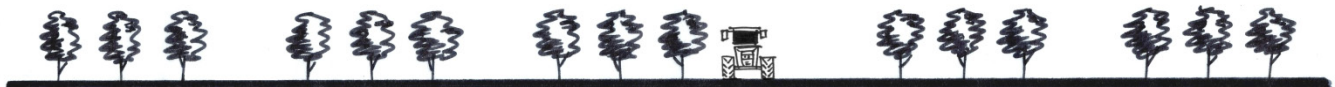
Figure 6. Field plantings should allow sufficient space for equipment access. A combination of field roads (narrower, turf-covered) and perimeter roads (wider, often gravel-covered) should be incorporated in the field design.
