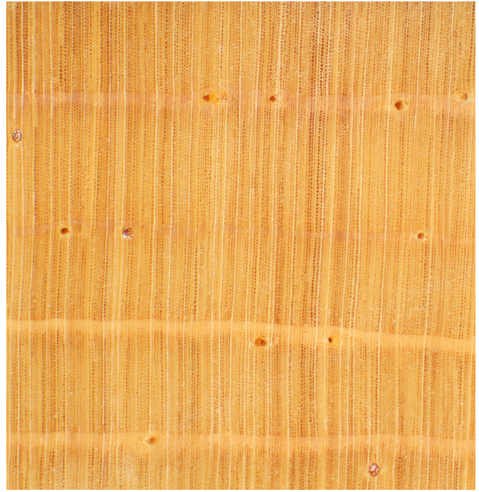
Figure 7-2. Eastern white pine ( Pinus strobus ), a medium-textured species. With a 10X lens, you can see that the surface is covered with tracheids, but it's practically impossible to distinguish any individual cell.
