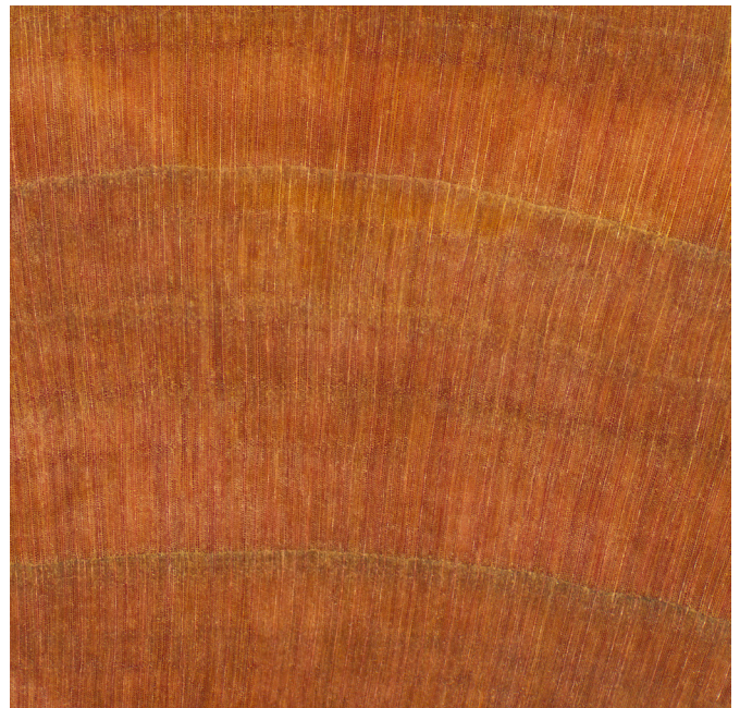
Figure 7-3. Eastern redcedar ( Juniperus virginiana ), a fine-textured species. Even with a 10X lens, it's impossible to distinguish any individual tracheids on this cross-section, and in fact you may not be able to distinguish any cells at all.
