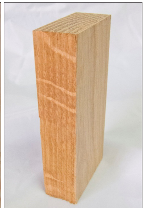
Figure 4-3. Red oak ( Quercus rubra ) (left) tangential face showing the cathedral grain on the tangential face formed by the large earlywood pores. The rays in oak are large enough to see easily, and they look somewhat like horizontal ribbons on the radial (quartersawn) face of the piece of white oak ( Quercus alba ) on the right. These ribbon-like patterns are referred to as ray fleck.
