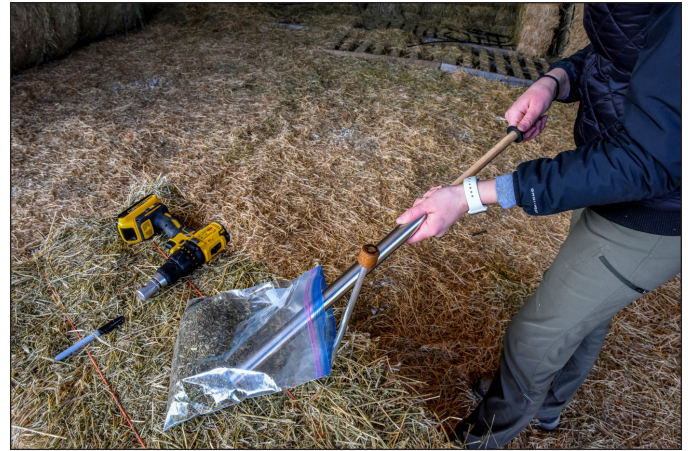
Figure 4. Some hay probes only hold one sample at a time and must be plunged into a bag or bucket between every sample.
