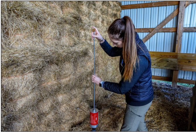
Figure 3. To avoid clogging the probe, use a plunger to clear the probe into the canister after each sample has been taken.
