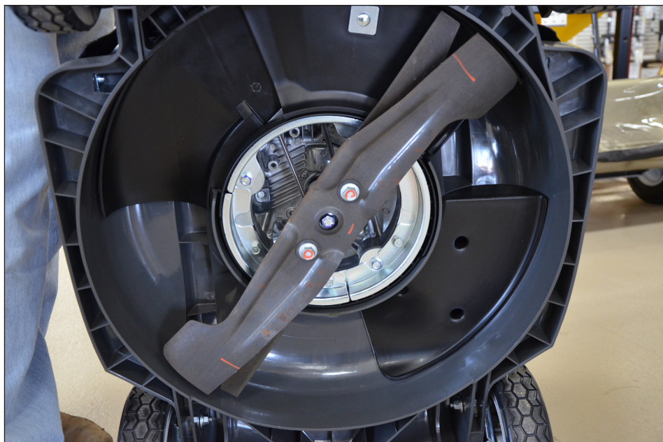
Figure 8. A mulching rotary mower showing a fully enclosed deck (lacking an exhaust chute) and a second blade to recut leaf blades.
