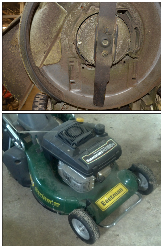
Figure 2. A rotary mower showing single blade (top) and a typical homeowner rotary mower (bottom).
