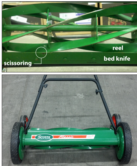
Figure 1. A reel mower showing scissoring action with reel to bedknife (top) and a standard lawn reel mower (bottom).
