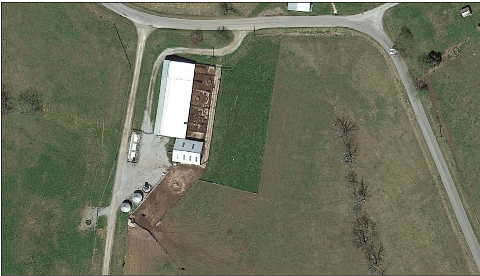
Figure 5. An aerial view of a vegetative treatment strip used to filter runoff from a feeding area.
