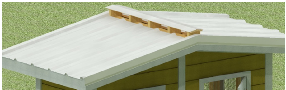
Figure 5. A continuous ridge vent, which ventilates both sides of the house.
