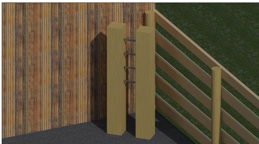
Figure 9. A corner of pen refuge can serve as a defensive structure for a producer in a livestock confinement area in the case of an emergency.
