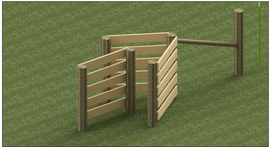
Figure 5. Livestock exclusion escape. Humans can make the sharp turn to enter and exit an area, but livestock cannot.
