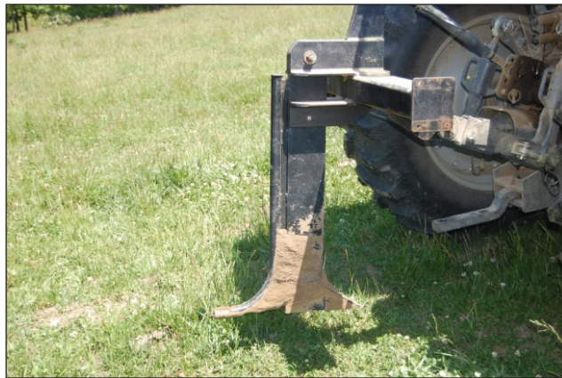
Figure 8. Ripping compacted soils along the contour of the slope can increase infiltration and reduce runoff. Photos by Dan Miller
