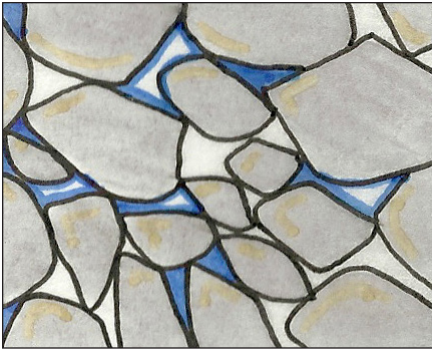
Figure 3. Pore space exists between individual particles of sediment and within sedimentary rocks.
